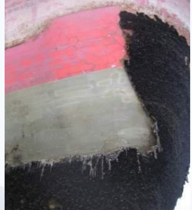
FPSO Terra Nova entering dry-dock after 7 years off Canada (no fouling control system)
